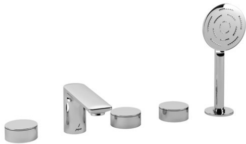
LAG-CHR-91287 5-hole bath tub mixer with hot & cold control cocks, spout, diverter & hand shower with 8mm dia. & 1.5m flexible tube
