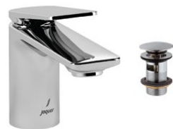
LAG-CHR-91011BCW Single lever basin mixer without popup waste, with 375mm long braided hoses & click clack waste (ALD-729)
