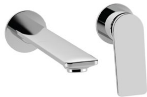
LAG-CHR-91231NK Exposed parts kit of single lever basin mixer wall mounted consisting of operating lever, cartridge sleeve, nipple, spout & two wall flanges (compatible with ALD-233NPSO & ALD-235NPSO)
